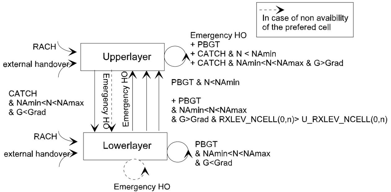
The handover that may occur to non preferred target cells due to the unavailability of TCH resources are indicated with dotted line arrows in the state diagram.
