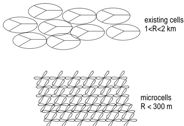
**Figure C.1: First scenario: microcells below existing cells**
