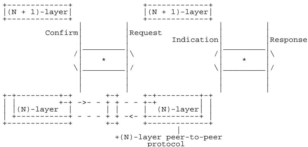
**Figure 5: Primitive action sequence for peer-to-peer communication**
